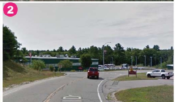
Lack of sidewalks and bicycle lanes on Great Hill Drive. Curves in the road also limit sight lines.
